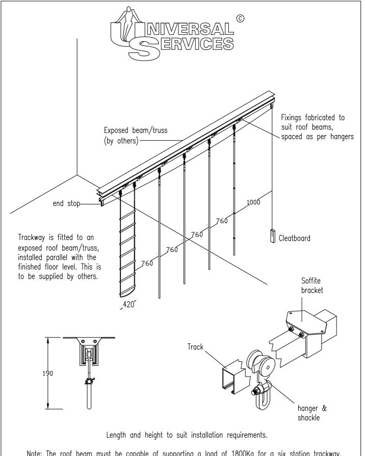
Note: The roof beam must be capable of supporting a load of 1800Kg for a six station trackway.
