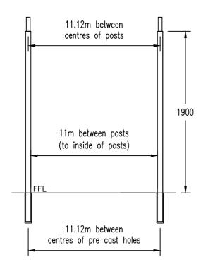
The telescopic socketed volleyball posts are supplied with heavy duty floor sockets. These must be professionally installed. Each socket requires a pre cast hole 152mm in diameter and 350mm in depth, to secure the socket an epoxy masonry adhesive must be used.
