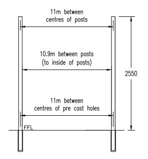
The socketed international volleyball posts are supplied with heavy duty floor sockets. These must be professionally installed. Each socket requires a pre cast hole 125mm in diameter and 320mm in depth, to secure the socket an epoxy masonry adhesive must be used.
