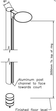
The international netball posts are supplied with heavy duty floor sockets and blanking caps, These must be professionally installed. The hole drilled for the socket needs to be 95mm in diameter and 310mm in depth, to secure the socket an epoxy masonry adhesive must be used. The concrete base must allow for drilling depth of 310mm.
