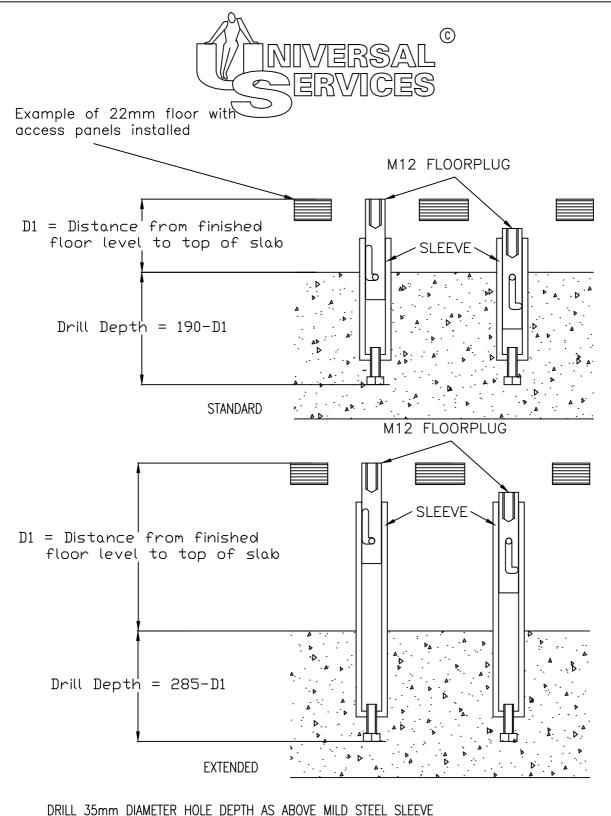
DRILL 35mm DIAMETER HOLE DEPTH AS ABOVE MILD STEEL SLEEVE 32mm DIAMETER STAINLESS STEEL FLOORPLUG 20mm DIAMETER THREADED TO SUIT M12 FASTENINGS
